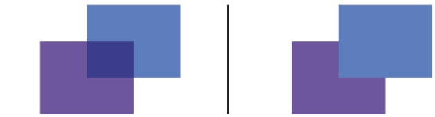
Left: Pantone 2665 C and Pantone 660 C on top with multiply transparency effect Right: Pantone 2665 C and Pantone 660 C set on overprint
