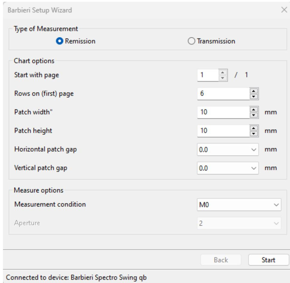
Click on **Start** to begin the measurement. Make sure that your chart complies with the layout requirements for the Spectro Swing (a corresponding preset is available in the **Export Chart** tool) and that the chart is correctly inserted into the device (short side first - the positioning marks must be on the left and bottom of the chart).
