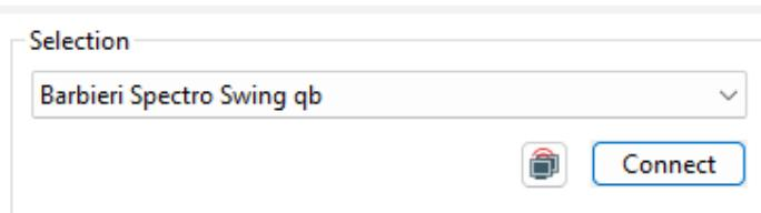
The device can be connected via USB or Ethernet. It is highly recommended to use the Ethernet connection as it provides higher transmission speeds. Click on the **Network** icon next to the **Connect** button to open the **Networking Setup**.
